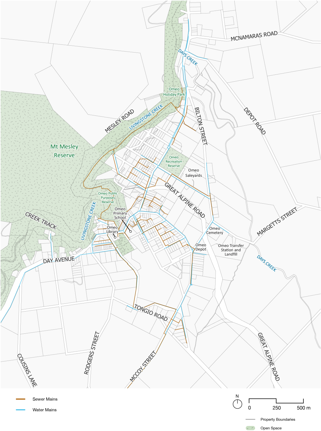
Figure 56: Omeo sewer and water servicing plan
