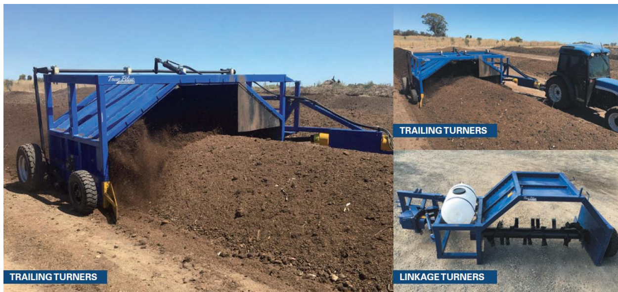
Figure 8: Example of suitable windrow turner (Source: True Blue Composters)
