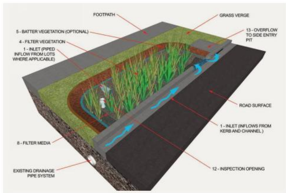
Figure 10 - Raingarden Components (Melbourne Water)
