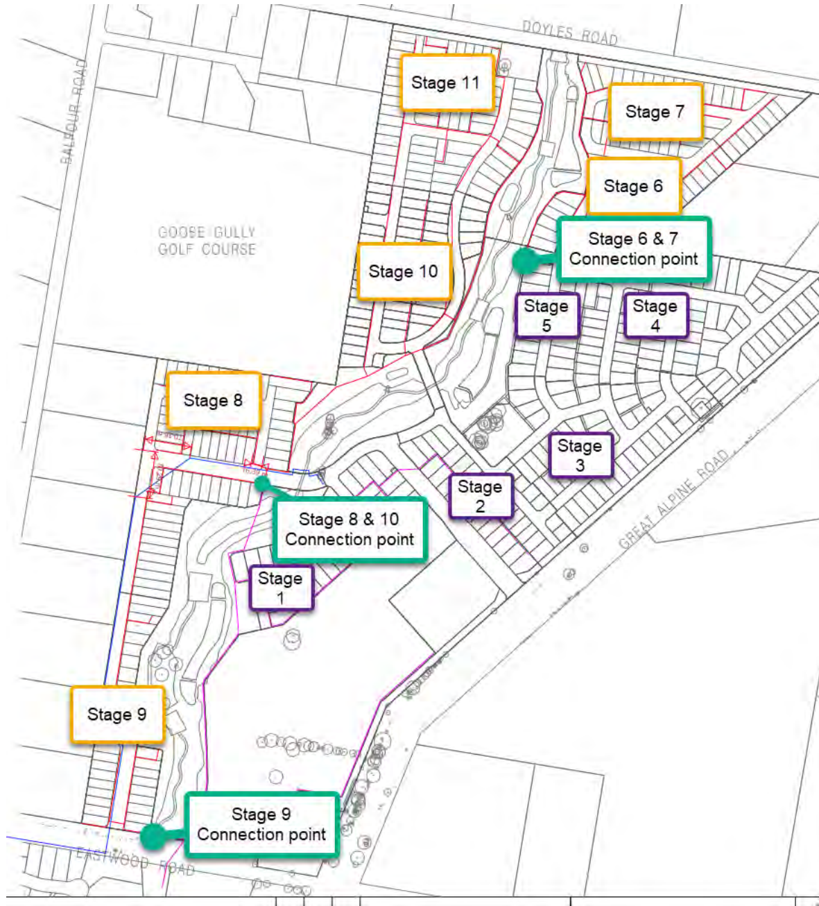
Figure 6 - Proposed Sewer Network (Source: Marshal)
